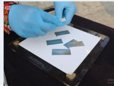
Dimensions: for each plate, Length & Width = 10 inch, Thickness = 6mm. Can cut TLC plates with a simple glass or paper cutter.
