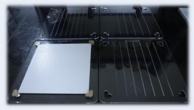
It is very safe, easy to use and time saving as no marking is needed. Can also be used for cutting of glass plates. ▶ Using this instrument we can cut a standard TLC plate (20cm\*20cm) into various sizes such as 2\*4cm, 2\*5cm, 2.5\*4cm, 2.5\*5cm, 3\*4cm, 3\*5cm, and many more bigger sizes
