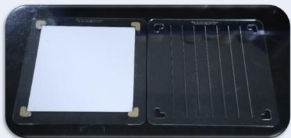
The device comes as combo of one base and three frames (with different number of groves) which can cut different sizes. This is very safe device as the cutter runs into groves so there is no hand cuts anymore while cutting the TLC plates.
